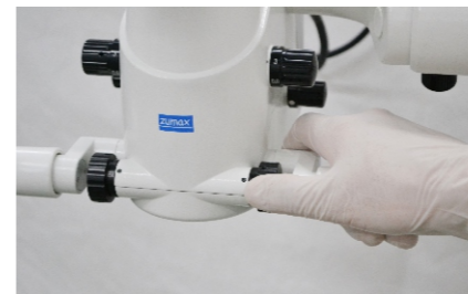
Adjust the fine focus knob
